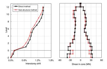
Figure 2. Comparison of the sub-structure method with the direct method.
