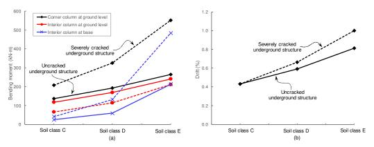
Figure 4. Results of NTLHA: (a) bending moment in columns, (b) drift at top of the building.
