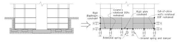
Figure 3. Conceptual model of the sub-structure method for modelling SSI.
