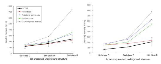
Figure 6. Elastic bending moment in the interior column at ground level. [Colour online].
