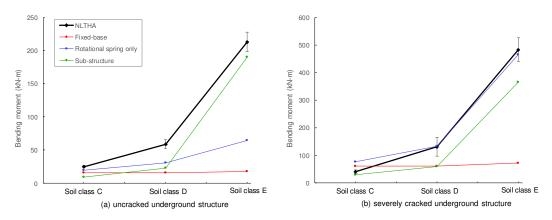
Figure 7. Elastic bending moment in the interior column at the base. [Colour online].
