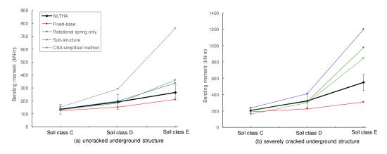
Figure 5. Elastic bending moment in the corner column at ground level. [Colour online].
